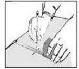
The straightedge could be a straight piece of lumber or piece of flooring. Alternatively, the first row can be face-nailed with finishing nails into the wood subfloor or spring nailed into a concrete subfloor.
